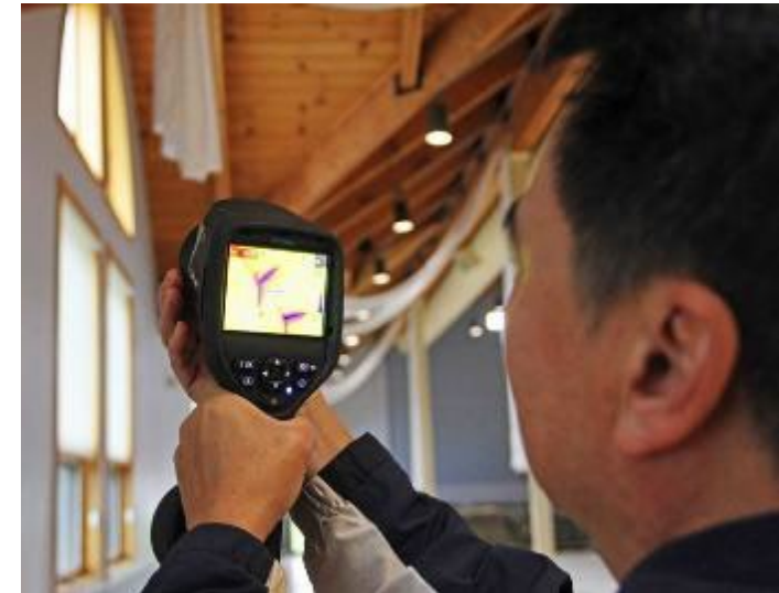
Building Envelope specialist utilize infrared cameras and other tools for comprehensive assessments
